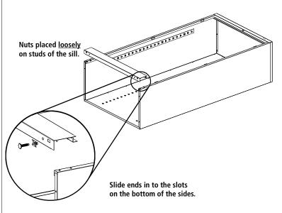
**7.** Place the rear flange of the bottom (Ref. No. 7) into the bottom lances of the back. The flange with two holes should face the front, hanging over the sill. Insert the bolts through the bottom and still with the head
