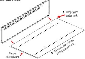
**4.** Attach the top (Ref. No. 5) to the unit by sliding the outer flange over the back of the unit and the side flange on the top over the side panel. The threaded studs should go
